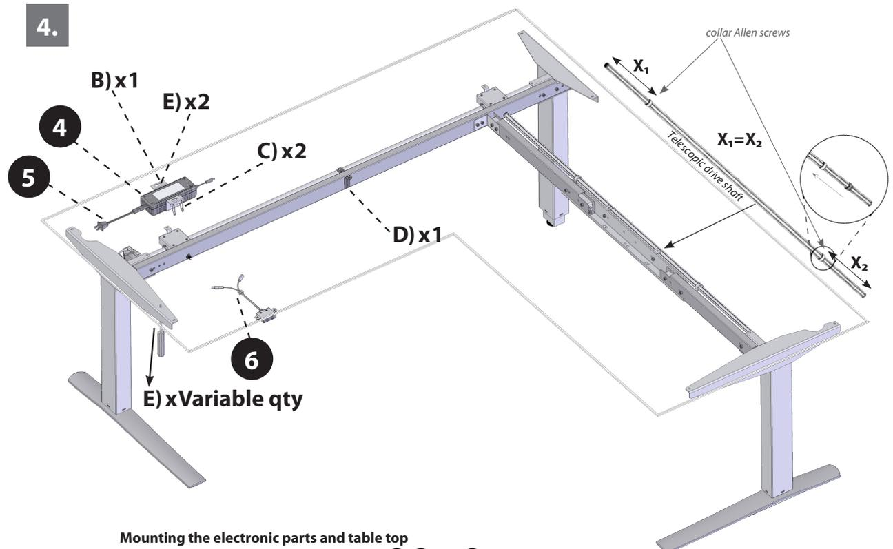
**Mounting the electronic parts and table top**
