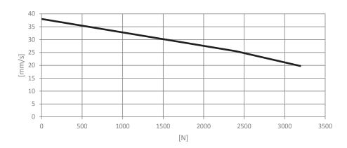
The above data are measured in connection with 2-4 DL10 lifting units and control box CBD4/CBD6S. The desk is driving upwards.
